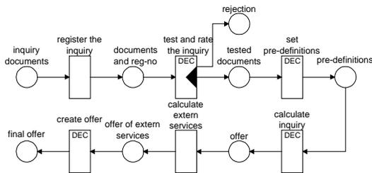
Figure 3: Sequence of Workout of Offers in Foundries
