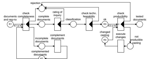
Figure 4: Subsequence “test and rate the inquiry”
