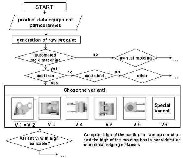
Figure 6: Part of an Algorithm for Generation of Raw Products for a Seiatu Molding Maschine
