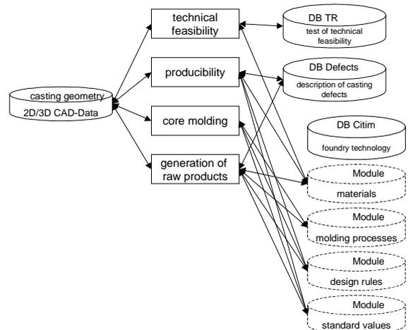
Figure 7: Databases of the Casting Design Process
