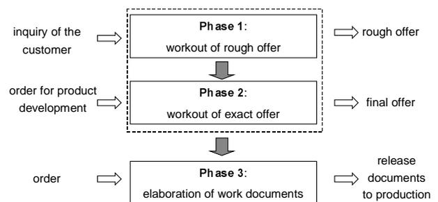
Figure 2: Phases of Work Scheduling in Foundries
